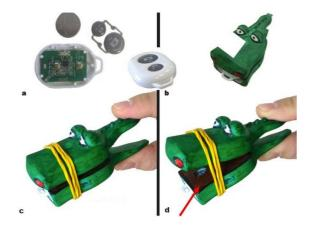
**Fig. 2** – Prototype of a pressure sensor for children hand rehabilitation [8].
